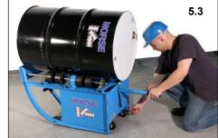
For compliance with safety regulations, the drum roller should be moved into an enclosure with safety interlock (image 5.4) before drum rolling is started.
